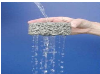
A stream of water is dispersed through a piece of pervious concrete.
